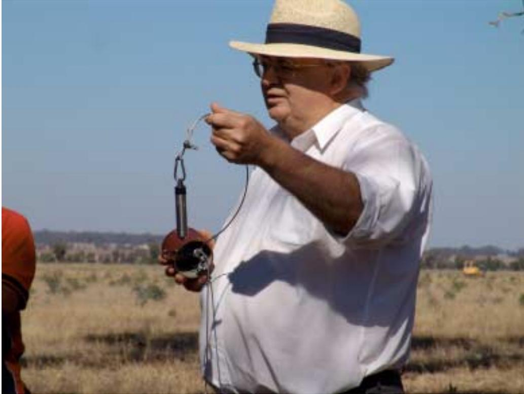
**Figure 1:** Phil Dyson holds an electronic datalogger that is located inside the groundwater bore and takes readings of the changes in the watertable every 30 minutes.
