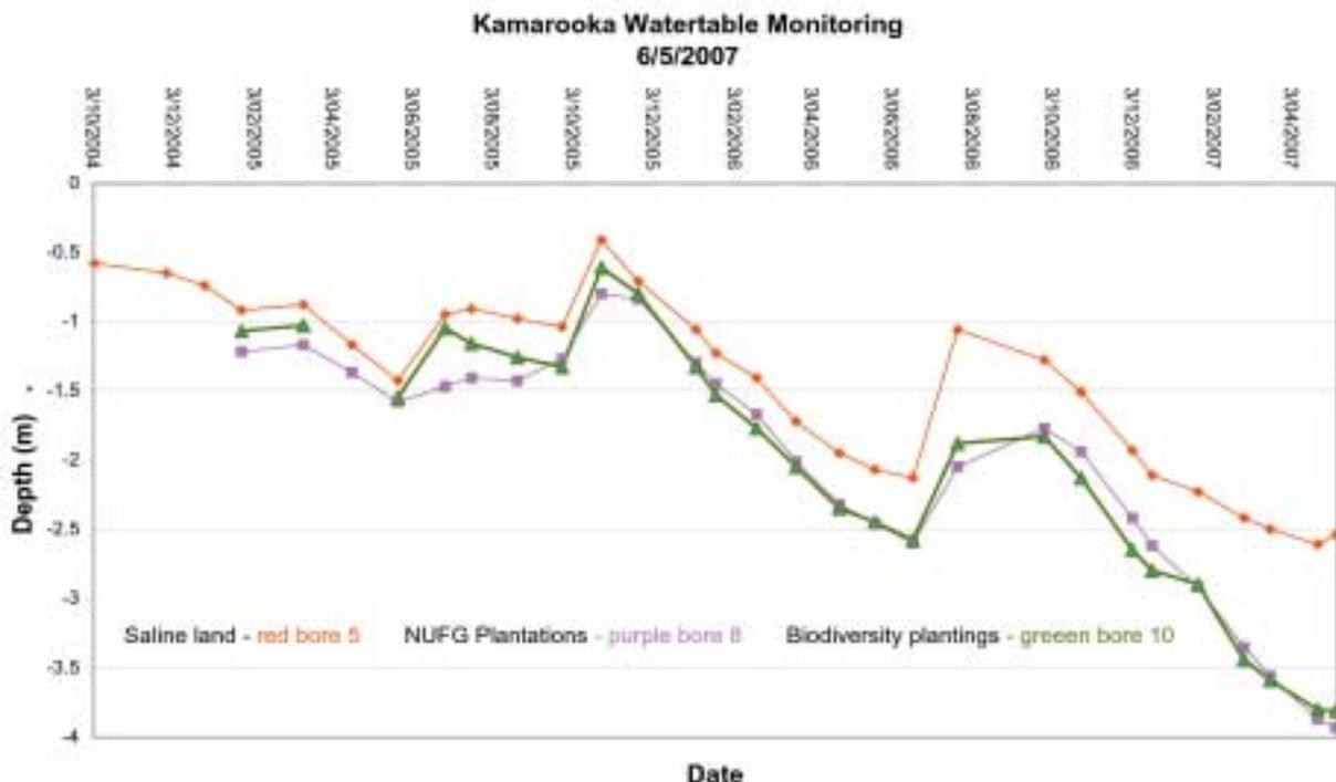
Figure 3: Bore data for the three treatments established as part of the Kamarooka Project
