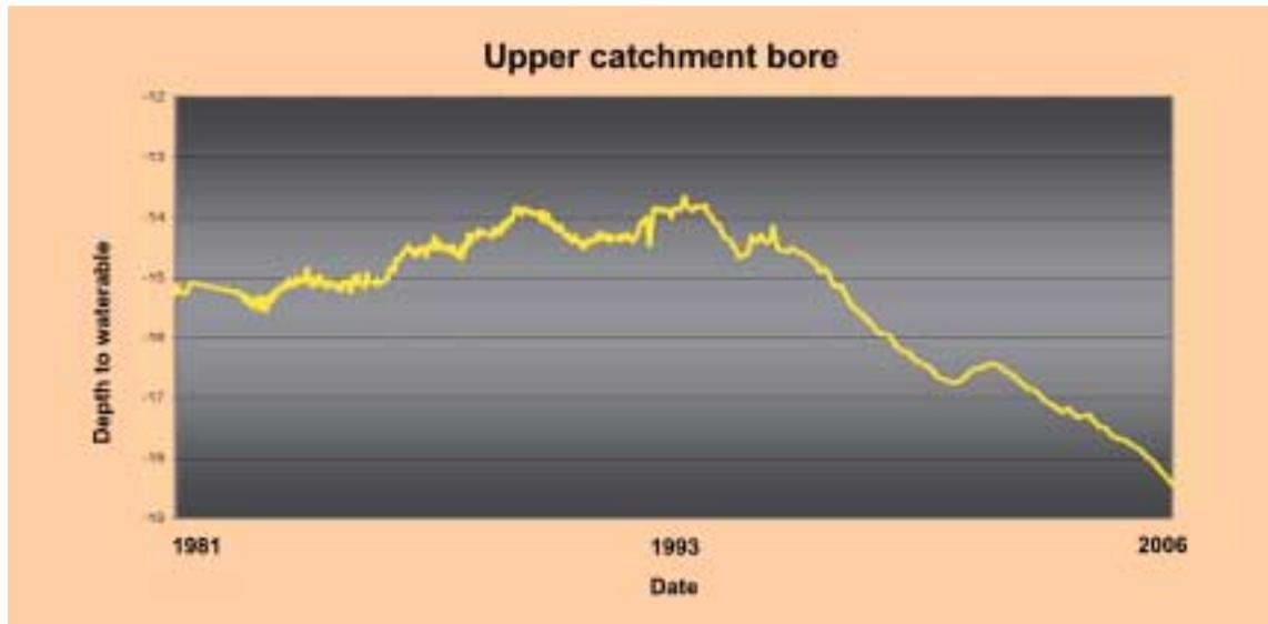
**Figure 2:** Decline in groundwater elevation in bore 72 (Upper Kamarooka catchment)
