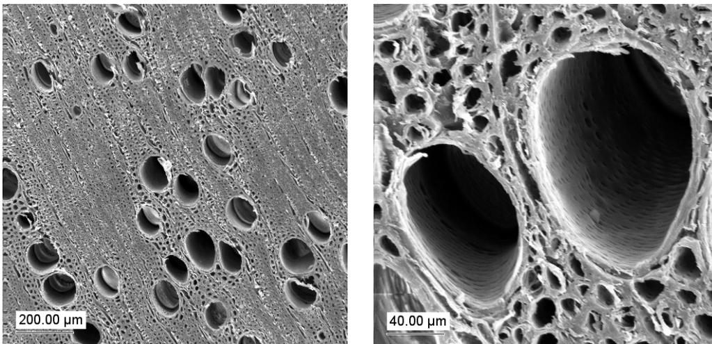
Figure 1 - Electron micrographs showing the xylem tubes in the stem of *E. cladocalyx* from the NUFG plantation at Kamarooka (courtesy of Dr. Sabine Wilkens - Latrobe University)
