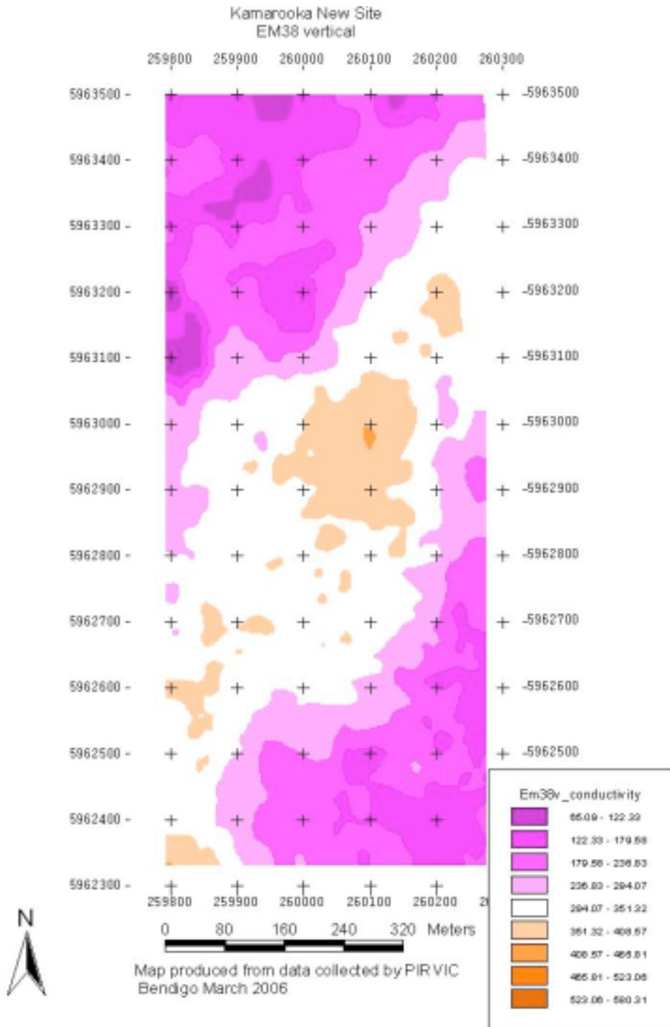
Figure 9 Image showing apparent electrical conductivity (salinity) - Kamarooka Stage 2 planting using EM-38 in vertical dipole mode.
