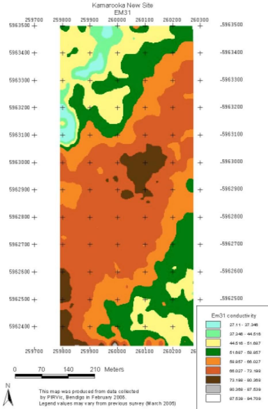
Figure 10 Image showing apparent electrical conductivity (salinity) - Kamarooka Stage 2 planting using EM-31.
