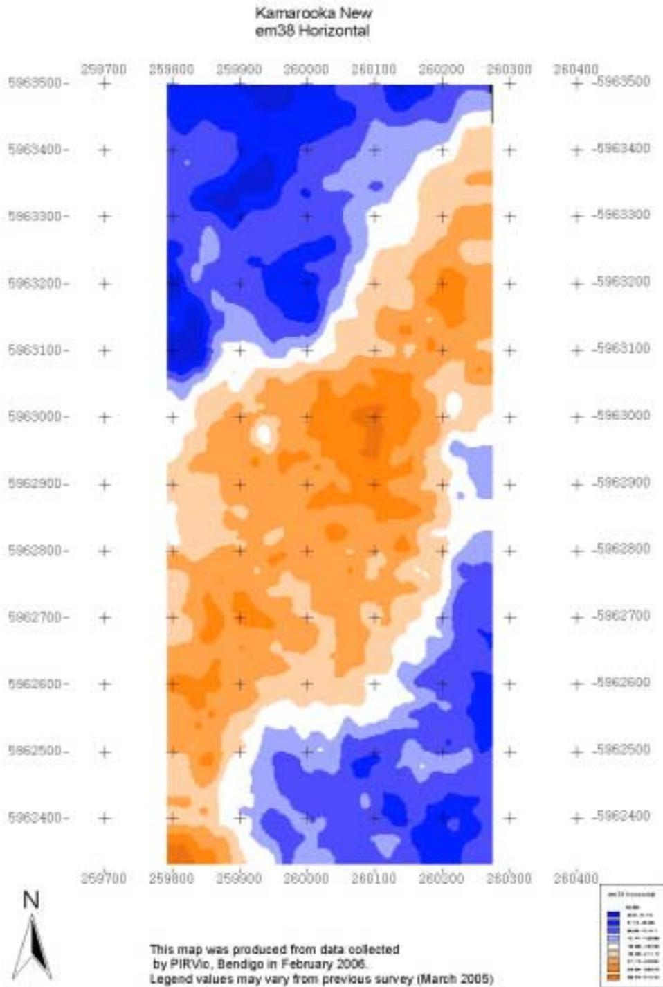
**Figure 8 Image showing apparent electrical conductivity (salinity) - Kamarooka Stage 2 planting using EM-38 in horizontal dipole mode.**
