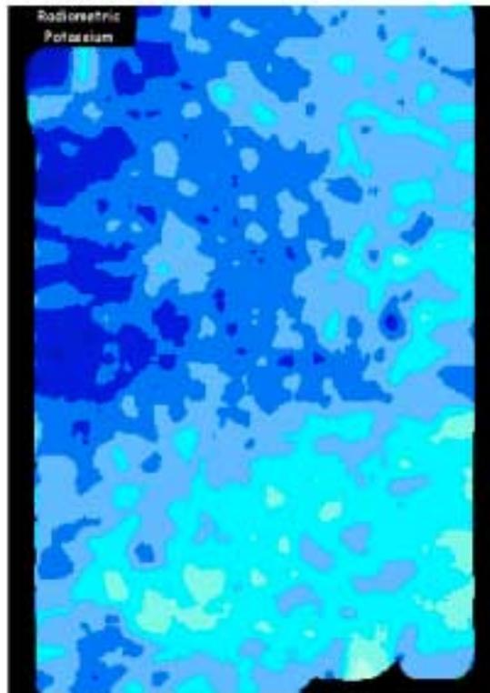
Figure 4 Image showing variation in radiometric Potassium.
